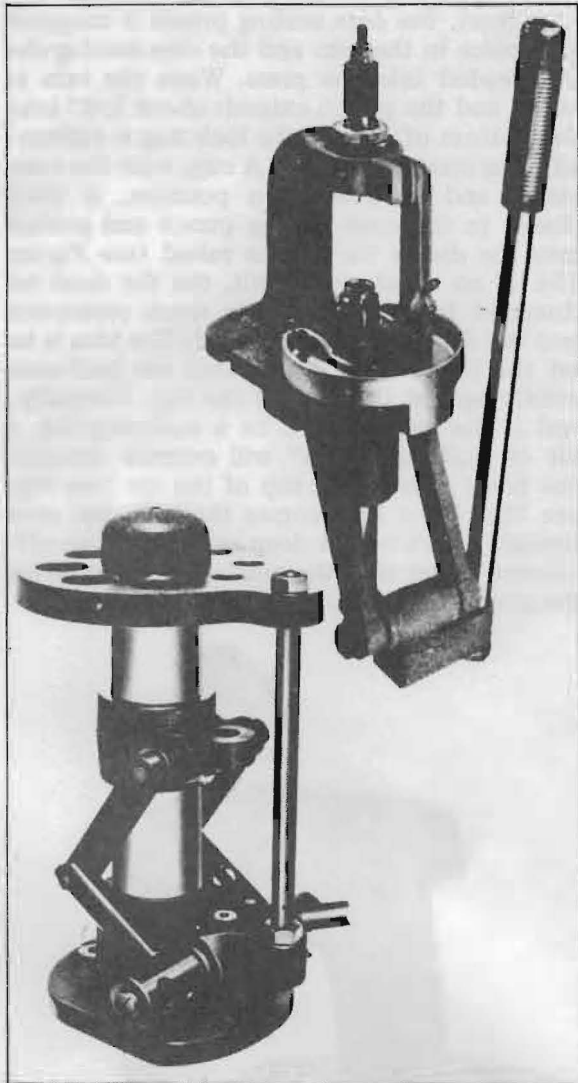
FIGURE 30 — Heavy-duty loading presses, such as the RCBS Rockchucker (top) and the Hollywood turret (shown with turret locking rod in place), are ideal for bullet swaging.
