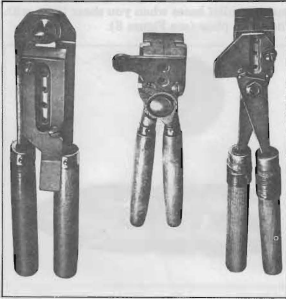
FIGURE 4 — Gang mold (left) has a sprue plate channel. Center, two-cavity mold has individual sprue holes and no channel. Mold at right has had a channel milled in by the owner.
