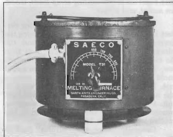
FIGURE 6 — When using gang molds, an electric furnace is desirable, to reduce the time lost between melts. The SAECO unit shown here holds 20 pounds of metal and has an automatic heat control.
