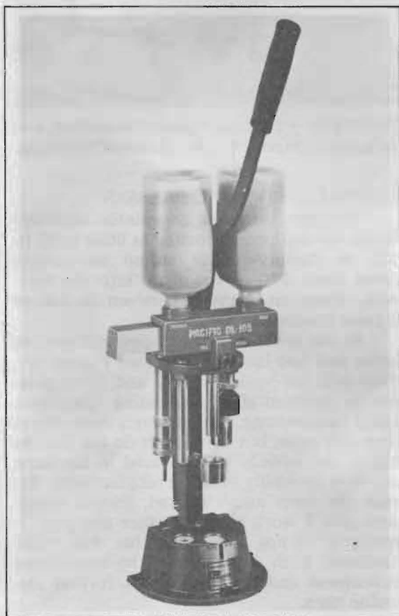
FIGURE 11 — The Pacific DL-105 is a good-quality single-stage press. The entire top assembly drops when the handle is operated.
