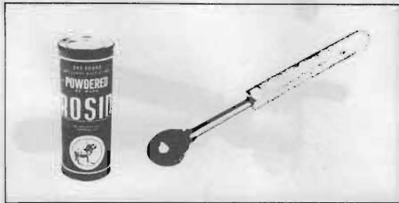
FIGURE 14 — Powdered rosin and a ladle are necessary for fluxing the molten metal. Rosin can also be used to prevent vise jaws from slipping on metal surfaces.
